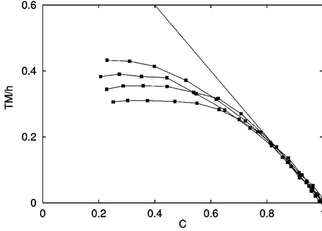
FIG. 1. Integrated response versus autocorrelations for  $T=0.5$  and  $\delta=2$ . The different curves correspond, from top to bottom, to waiting times  $t_w=2^5, 2^7, 2^9, 2^{11}$ . The straight line corresponds to the FDT relation  $TM/h=1-C$ .
