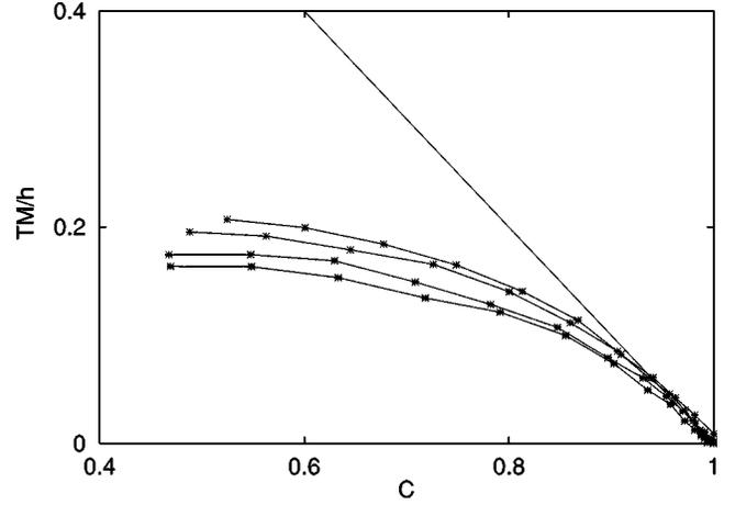
FIG. 2. Integrated response versus autocorrelations for  $T=0.5$  and  $\delta=4$ . The different curves correspond, from top to bottom, to waiting times  $t_w=2^5, 2^7, 2^9, 2^{11}$ . The straight line corresponds to the FDT relation  $TM/h=1-C$ .
