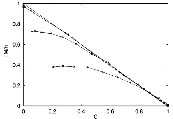
FIG. 3. Integrated response versus autocorrelations for  $t_w=2^7$  and  $\delta=2$ . The different curves correspond, from top to bottom, to temperatures  $T=1, 0.7, 0.5$ . The straight line corresponds to the FDT relation  $TM/h=1-C$ .
