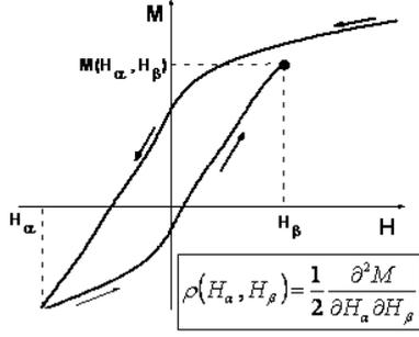
Fig. 1. Scheme of a FORC measurement and involved variables.
