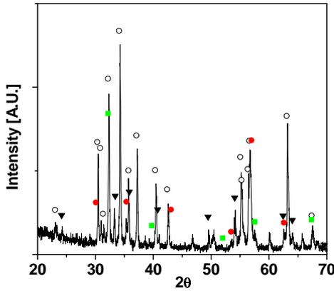
Fig. 2. X-ray diffraction pattern. Open circles:  $\text{BaFe}_{12}\text{O}_{19}$ , solid (red) circles:  $\text{CoFe}_2\text{O}_4$ , solid (black) triangles:  $\text{Fe}_2\text{O}_3$ , solid (green) squares:  $\text{LaFeO}_3$
