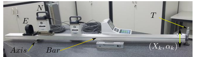
Fig. 6: Experience with electronic level and autocollimator.
