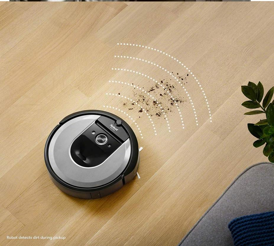
Robot detects dirt during pickup
