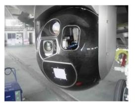
video cameras, an infrared range-finder, a laser platform, commando, display & recording units and inertial unit assisted by a GPS receiver.
