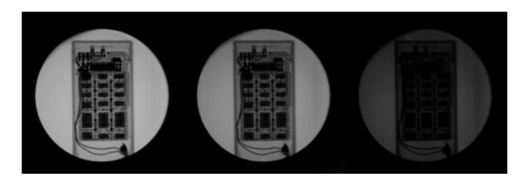
Fig. 2 Luminous-screen image of a pocket calculator (photographed using a digital camera) at maximum tube high voltages and different emission currents.
