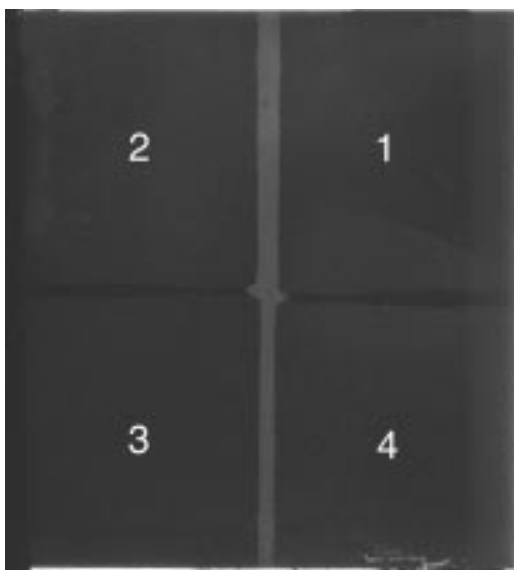
Fig. 5 Fogging of x-ray film at a constant product of I \cdot \Delta t Field 1: I = 0.25 mA, \Delta t = 5 s, Field 2: I = 0.50 mA, \Delta t = 10 s, Field 3: I = 0.72 mA, \Delta t = 14 s, Field 4: I = 1.00 mA, \Delta t = 20 s
