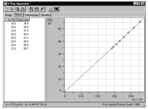
Fig. 4 Sections from the diffraction spectra of x-radiation for the tube high voltages *U* = 22, 24, 26, 28, 30, 32, 34 and 35 kV (from right to left) with best-fit straight line for determining the limit
