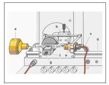
Fig. 3 Experiment setup in Bragg configuration
