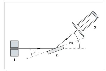
Fig. 2 Schematic diagram of diffraction of x-rays at a monocrystal and 2θ coupling between counter-tube angle and scatter-ing angle (glancing angle)
