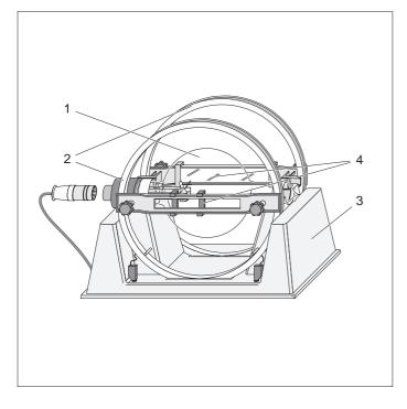
The fine beam tube (555 571) is used in conjunction with the Helmholtz coils with holder and measuring device (555 581) to investigate the deflection of electron beams in electrical and magnetic fields, particularly the determination of the specific electron charge e/m.
