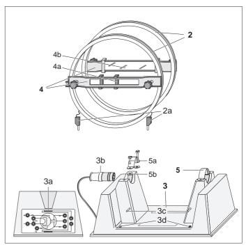
Pair of Helmholtz coils 2 4-mm plug (2a)
