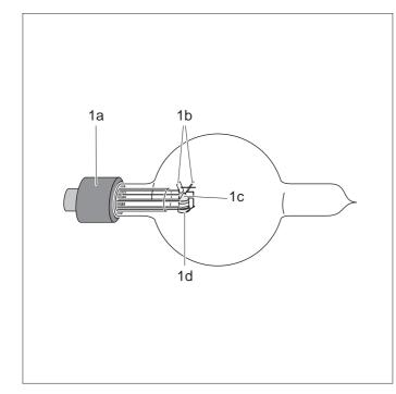
1 Fine beam tube base (1a), deflection plates (1b), anode (1c), cathode, Wehnelt cylinder (1d)
