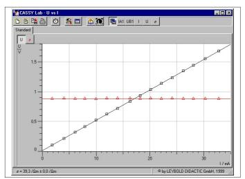
5.2 Hall voltage  $U_{\rm H}$  as a function of the magnetic flux density B
