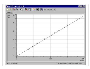
5.5 Voltage drop U and conductivity  $\sigma$  as a function of the magnetic flux density B
