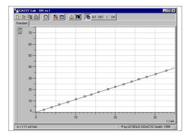
5.4 Voltage drop  $\emph{U}$  and conductivity  $\sigma$  as a function of the cross-current  $\emph{I}$  through the Ge crystal
