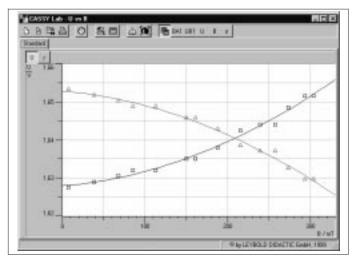
5.6 Voltage drop U and conductivity  $\sigma$  as a function of the absolute temperature T
