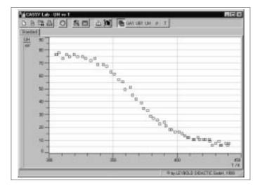
5.4 Voltage drop U and conductivity  $\sigma$  as a function of the cross-current *I* through the Ge crystal
