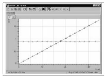
5.5 Voltage drop U and conductivity  $\sigma$  as a function of the magnetic flux density B
