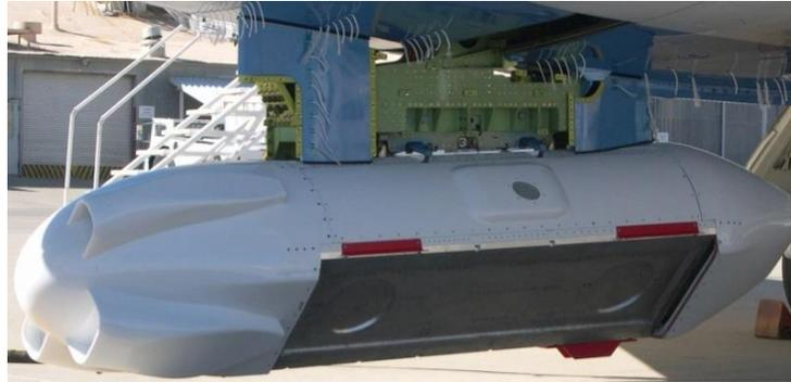
**Figura B.5: Sensor Aerotransportado UAVSAR<sup>9</sup>**
