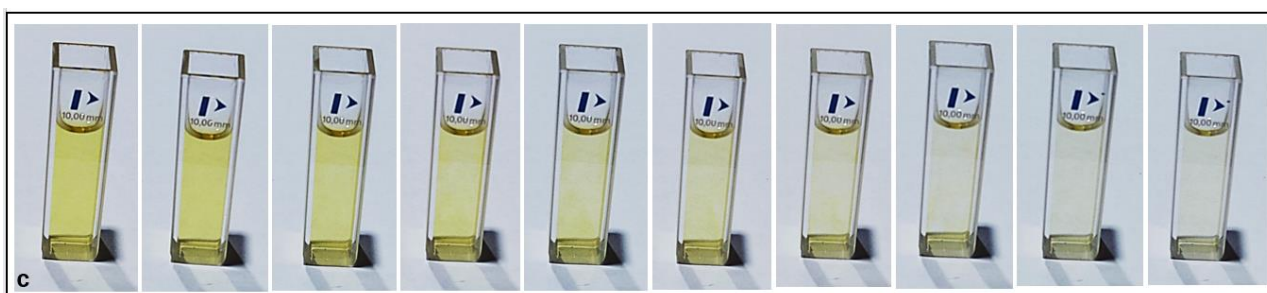
Figure 4. a) Response of AgNPs@starch at 400 nm upon addition of Cr(VI) in the range 0 to 84 \mu\text{M} . b) Calibration curve of Absorbance vs \mu\text{M} Cr(VI). c) Solution color change upon AgNPs@starch aliquots addition.
