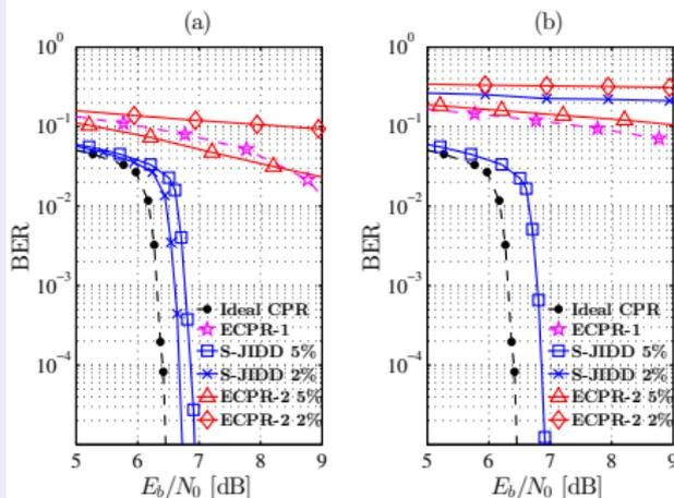
Performance comparison between two state of the art Carrier Phase Recoveries (ECPR-1 and ECPR-2) and the proposed Joint Iterative Demapper and Decoder (JIDD) with integrated carrier phase recovery.
