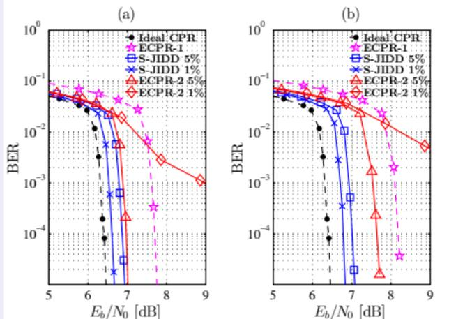
Performance comparison between two state of the art Carrier Phase Recoveries (ECPR-1 and ECPR-2) and the proposed Joint Iterative Demapper and Decoder (JIDD) with integrated carrier phase recovery.
