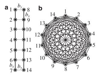
FIG. 2. Panel (a) shows the coupling network of a spin ladder. Panel (b) contains the coupling network of a spin star in which all the spins interact with each other.
