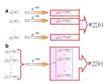
FIG. 1 (color online). (a) Schemes of the quantum evolution of an ensemble and (b) a pure state. Each  $|\Psi_i^m\rangle = |\psi_m\rangle \otimes |\Psi_i\rangle$  contains a complete base,  $|\Psi_i\rangle$ , of the M-m spins.
