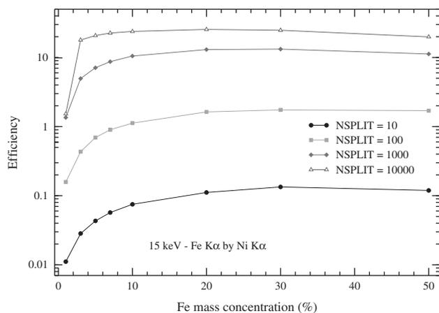
**Figure 3.** Efficiency of the Monte Carlo algorithm for the assessment of Fe-K $\alpha$  secondary intensity induced by Ni-K $\alpha$  as a function of Fe concentration for 15 keV incident electrons for different NSPLIT values.
