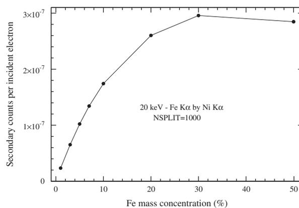
**Figure 4.** Fe-K $\alpha$  secondary intensity enhanced by Ni-K $\alpha$  as a function of Fe mass concentration for beam electrons of 20 keV.
