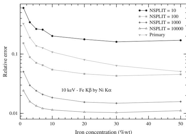
**Figure 5.** Relative errors for Fe-K $\beta$  intensity enhanced by Ni-K $\alpha$  at 10 keV as a function of Fe concentration for different NSPLIT values. Uncertainties for primary Fe-K $\beta$  intensity are also shown for comparison.
