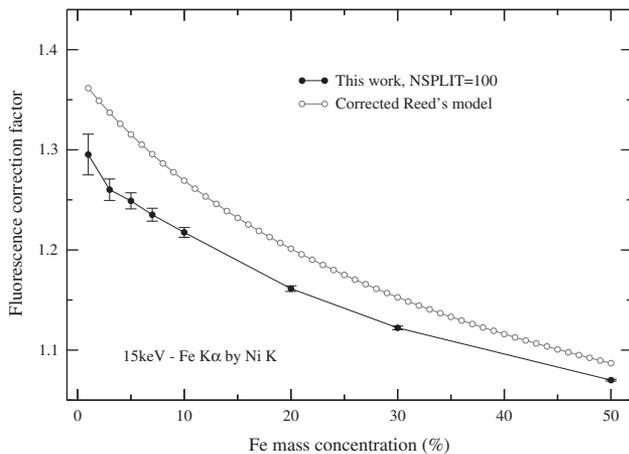
**Figure 1.** Comparison of the present Monte Carlo simulation for the fluorescence correction factor with the modified Reed’s model of Venosta & Castellano (2013) for an electron beam energy of 15 keV as a function of Fe mass concentration.
