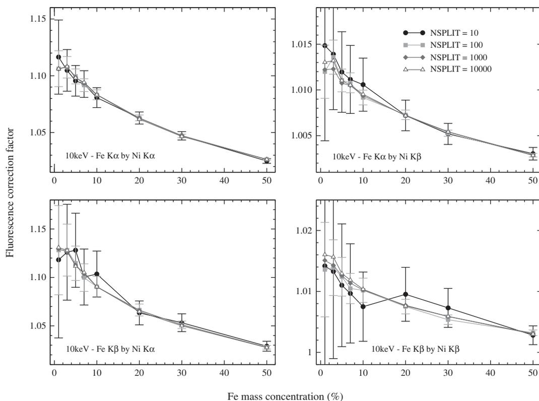
**Figure 2.** Fluorescence correction factor for an electron beam energy of 10 keV as a function of Fe mass concentration: Fe-K $\alpha$  by Ni-K $\alpha$ , Fe-K $\alpha$  by Ni-K $\beta$ , Fe-K $\beta$  by Ni-K $\alpha$ , and Fe-K $\beta$  by Ni-K $\beta$ . Only error bars for NSPLIT 10 and 100 are displayed.
