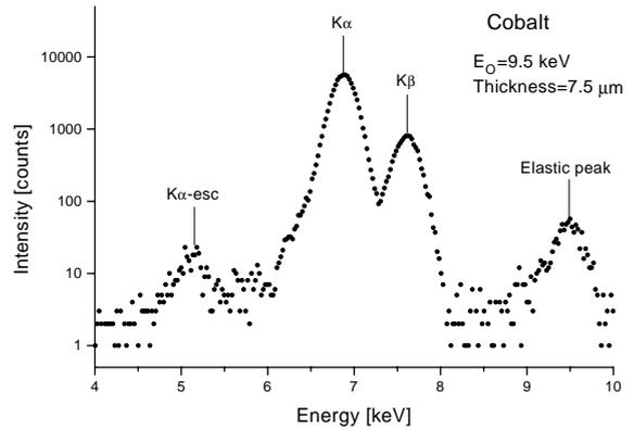
Fig. 2. Cobalt spectrum acquired for an incident beam energy of 9.5 keV. Notice the very low background only appreciable with logarithmic scale.
