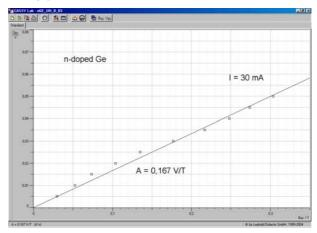
Fig. 5: Hall voltage  $U_{\text{H}}$  as function of the magnetic field B for I = 30 mA.. The straight line with slope A corresponds to a fit according equation (I).
