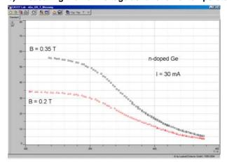
Fig. 6: Hall voltage  $U_H$  as function of the temperature T for  $I=30\ mA$  and different magnetic fields B.
