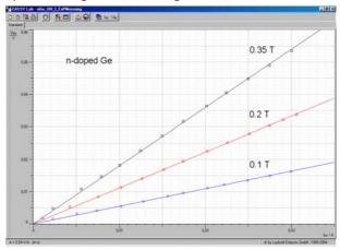
Fig. 4: Hall voltage U<sub>H</sub> as function of the current I for different magnetic fields. The straight lines correspond to a fit according equation (I).
