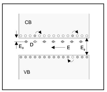
Fig. 2: Simplified diagram of extrinsic (left) and intrinsic conduction (right) under influence of an electric field E: Incorporating of dopants (donors D) into the crystal lattice creates negative charge carriers (electrons) in the conduction band (CB). With increasing temperature the thermal energy of valence electrons increases allowing them to breach the energy gap E<sub>g</sub> into the conduction band (CB) leaving a vacancy called hole in the VB.
