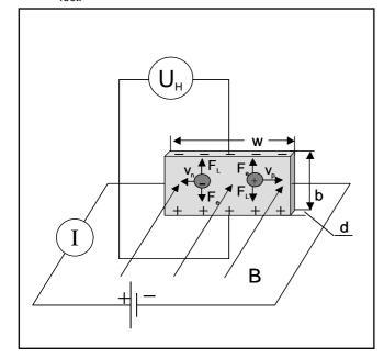
From equation (II) follows: The polarity of predominant charge carriers can be determined from the Hall coefficient  $R_{\rm H}$  if the directions of the current I and magnetic field B are known. The thinner the conducting strip the higher the Hall voltage.
