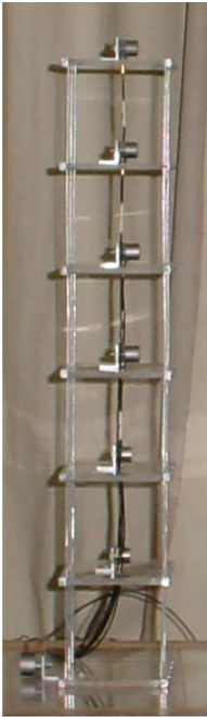
Figure 14. One bay, six-storeys high aluminum 3D frame model tested by Amani 2007.
