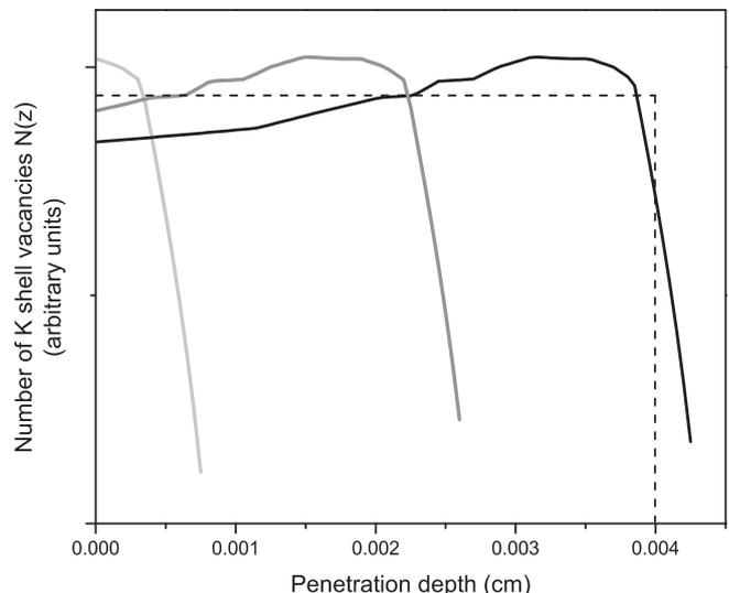
**Fig. 2.** Number of K-shell vacancies as function of depth for several incident energies: 2 MeV (black solid line), 1.5 MeV (gray solid line) and 0.7 MeV (light gray solid line). The dashed line is the step function that approximates the 2 MeV situation.
