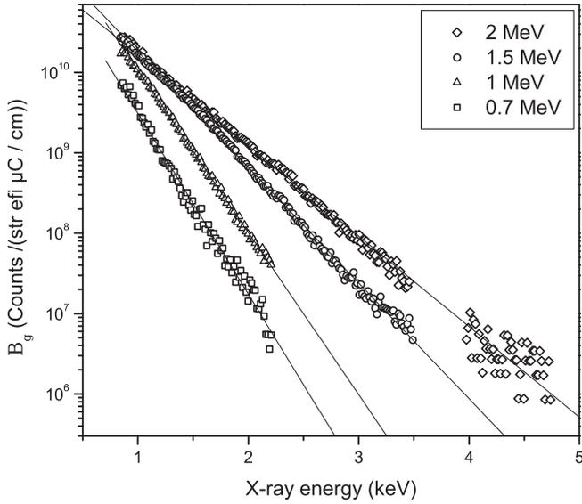
Fig. 3. Bremsstrahlung spectra of carbon generated within the sample for several incidence proton energies. Only four curves are plotted for clarity.
