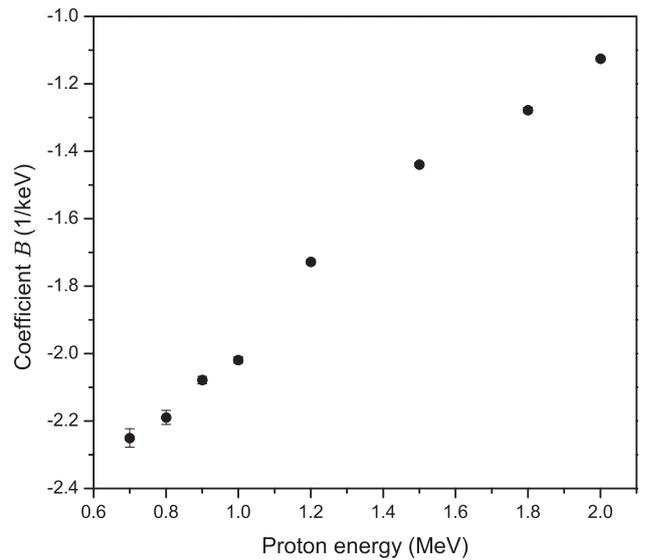
Fig. 4. Coefficients  $A$  and  $B$  of Eq. (4) as function of incident energy. Error bars are taken from fitting deviations and when missing they are smaller than the point size.
