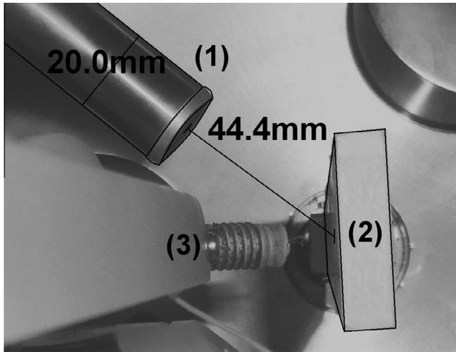
**Fig. 1.** Photography of the experiment set up. (1) EDS detector, (2) sample holder and (3) proton beam.
