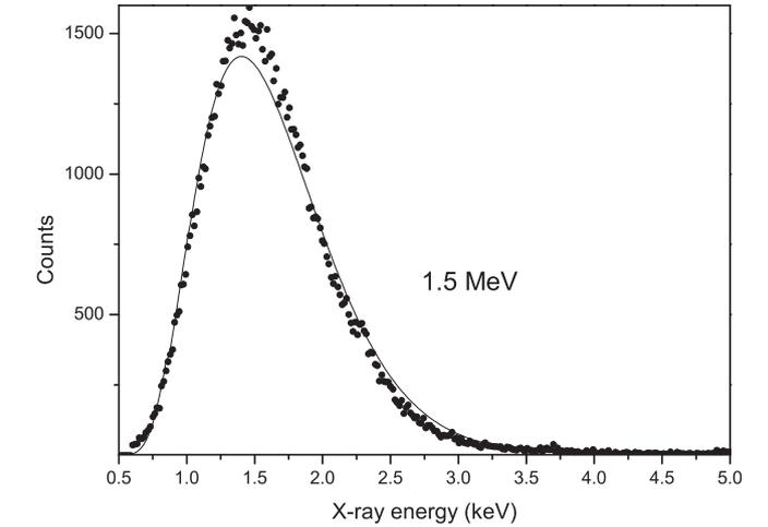
Fig. 5. Bremsstrahlung spectrum produced by 1.5 MeV protons in a bulk carbon target. Dots: experimental spectrum measured with a Si(Li) detector; line: prediction given by the proposed model.
